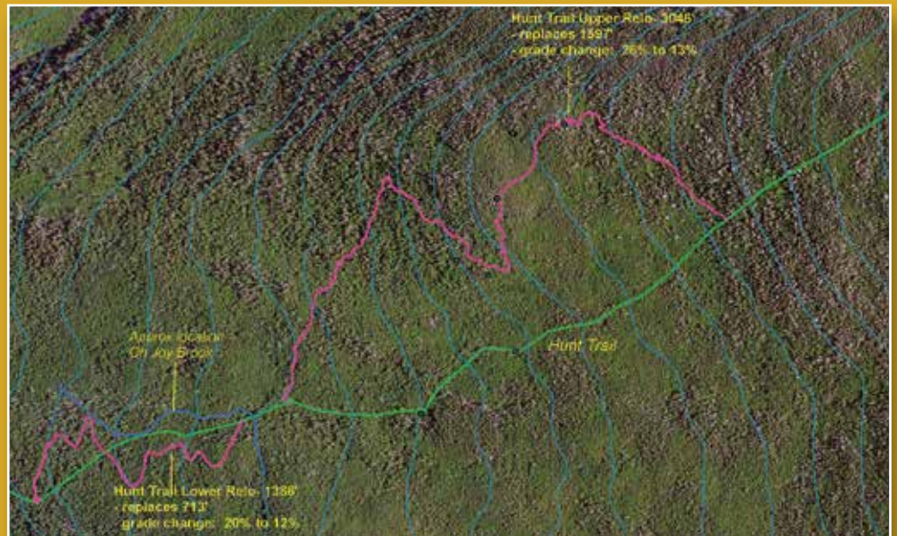
Baxter State Park is planning an ambitious schedule of trail relocations over the next decade through the Trautmann Trail Improvement Initiative. One of the next projects in the lineup is a relocation of two heavily eroded segments of the Hunt Trail above Katahdin Stream Falls. The new routes, shown in pink on this map, will offer a lower grade and improved treadway.
